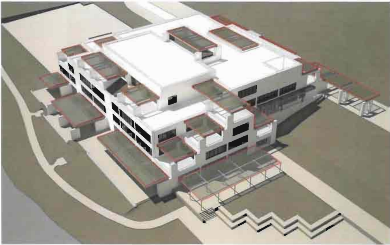
Locations of Potential New Rain and Sun Screens (red dashed outlines shown for clarity. New screens at all hidden trellises allowable also.)
